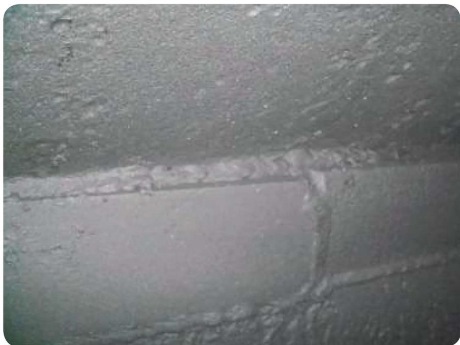
**FIGURE 4** White metal blast, as defined in NACE No. 1/SSPC-SP 5.
